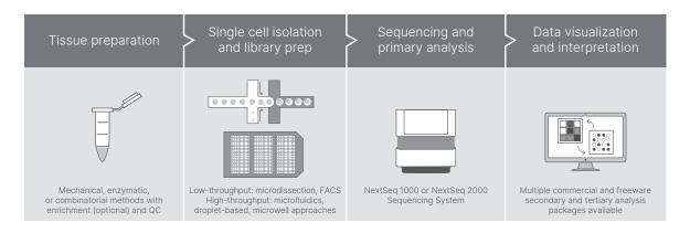
Figure 2: NextSeg 1000 and NextSeg 2000 scRNA-Seg workflow—The NextSeg 1000 and NextSeg 2000 Seguencing Systems are part of an integrated NGS workflow that proceeds from initial tissue preparation through single-cell isolation and library preparation, sequencing and primary analysis, and data visualization and interpretation.
